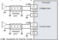
\*1 For analog input wiring, use shielded twisted-pair cables (double-core type). Separate them from other power lines or lines which are sensitive to industria.
